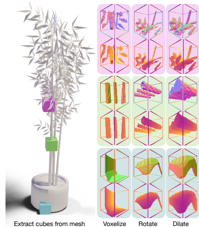
Figure 5.12: Training data for Nerfbusters diffusion model. Given a mesh, we extract local cubes scaled 1-10% of the mesh size. We voxelize these cubes with resolution 32^3 , and augment them with random rotations and random dilation.
