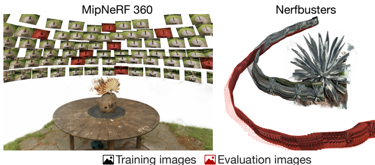
Figure 5.10: Evaluation protocols. Current evaluation of NeRFs (e.g., MipNeRF 360) measures render quality at every 8th frame of the captured (training) trajectory, thus only testing the model’s ability to render views with small viewpoint changes. In contrast, we propose a new evaluation protocol, where two sequences are captured of the same scene: one for training and one for evaluation. Please see the supplementary material for plots showing the training and evaluation sequences for various NeRF datasets, including our proposed Nerfbuster Dataset.
