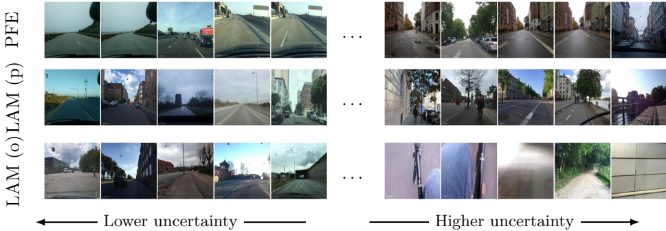
Figure 3.8: Images with lowest and highest variance for PFE, post-hoc LAM, and online LAM across MSLS validation set. LAM reliably associates high uncertainty to images that are blurry, are captured facing the pavement, or contain vegetation. These images do not contain features that are descriptive of a specific place, making them especially challenging to geographically locate.
