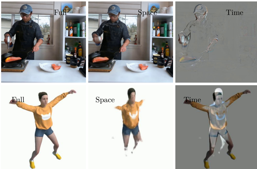
Figure 5.7: Decomposition of space and time. K-planes (left) naturally decomposes a 3D video into static and dynamic components. We render the static part (middle) by setting the time planes to the identity, and the remainder (right) is the dynamic part. Top shows the flame salmon multiview video [Li+22a] and bottom shows the jumping jacks monocular video [Pum+21].
