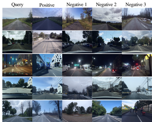
Figure 6: Triplets with multiple negatives. Hard-negatives are mined during training using our proposed sub-caching methodology. For each query-positive pair, the negatives that most violate the triplet constraint, \|q-p\|_2^2 + m < \|q-n\|_2^2 , are chosen. Here q , p , n refer to the cached embeddings for the query, positive and negative images. m is the margin.
