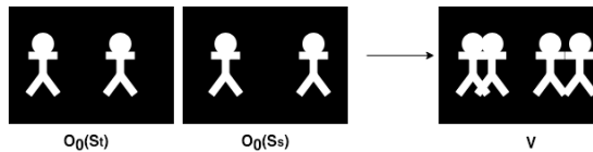
Figure 3.5: Shows an example of Equation 3.16 where the static background is obtained for two images. The union of these two masks gives the scenery that is static throughout the entire sequence. White indicate 0 (thus dynamic object) and black indicates 1 (thus static).
