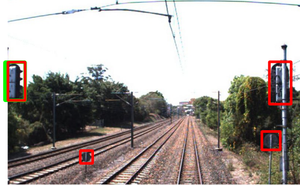
Figure 2.13: Shows an image crop of 500 \times 800 pixels taken from the center of the panoramic image. The red bounding boxes show the used bounding boxes. The green bounding box shows the original bounding box. From this figure it is seen that one bounding box has been cropped. The choice of crop means that we do not have to deal with the distortion observed in Figure 2.7.
